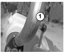
The green LED (1) will be illuminated as soon as operating frequency has been reached, the green LED indicates that the COMPATROL® compaction measurement system is ready for operation.
