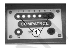
If all LEDs (1) are illuminated then compaction must be stopped immediately.
