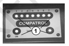
If the red and green LEDs (1/2) are illuminated, then the material cannot be compacted. The substrate should be replaced with material that can be compacted.
