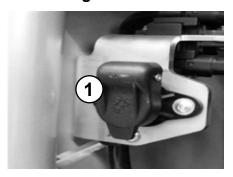
Insert plug (1) into the charging socket.
