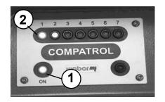
During the compaction work compaction is continuously measured and displayed visually via the yellow LEDs 1-7 (1). Maximum possible compaction is reached as soon as there is no noticeable increase in the illuminated LEDs.
